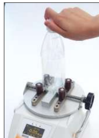
↑Opening PET bottle cap torque test
