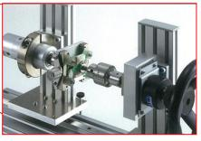
Torque-Angle Measurement of a small switch
